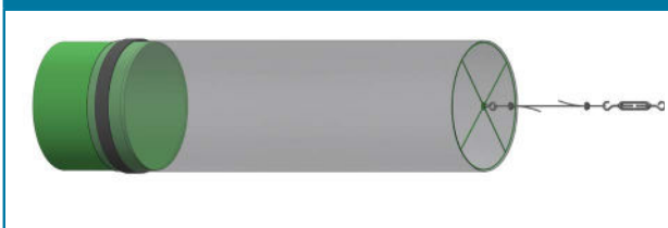
Anchored into the wall in the axis of the diffuser
